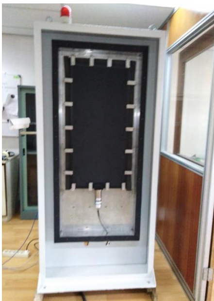
Gambar 7. Detektor BC408 didalam pilar
