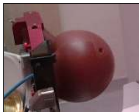
Gambar 3. Fantom ELEKTA solid water spherical phantom
